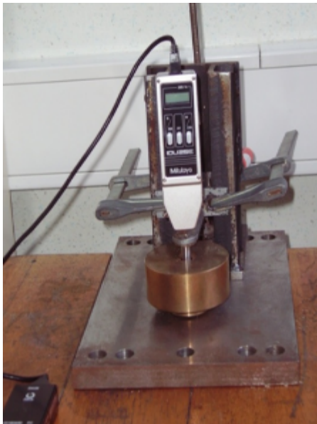
Figure 6 : The micrometer used for the measurement of the veneer thickness
