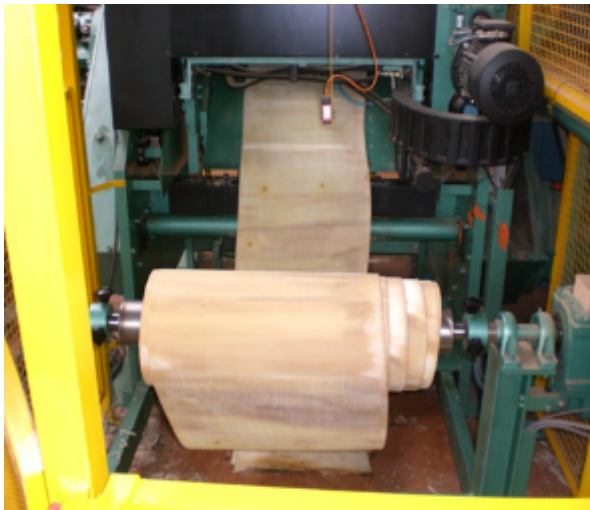
Figure 1: The peeling lathe of LaBoMaP.
