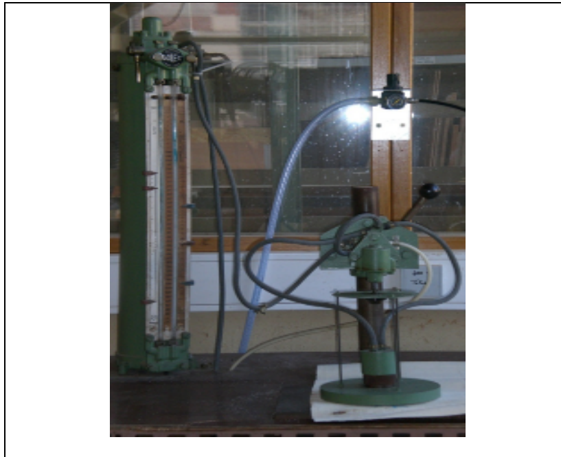
Figure 8: The leakmeter device used for roughness evaluation.
