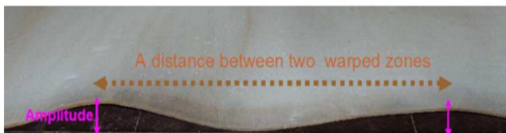
Figure 3: The curlup measurements.
